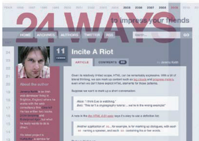
FIG 5.01: The “about the author” text in this screenshot should be marked up with footer , not aside .
